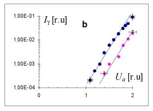
Fig.2. The light radiation intensity ( $I_{\gamma}$ ) vs RF power ( $U_a$  is the loop signal) for two types of cavities: space homogeneous (a) and space inhomogeneous (b) RFQ.
