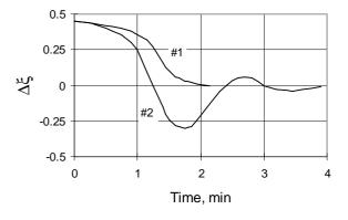
Figure 1:  $\xi(t)$ -transient in the tank #2 after repeated channel turn-on.  $\Delta \xi = \xi(t) - \xi_0$ .
