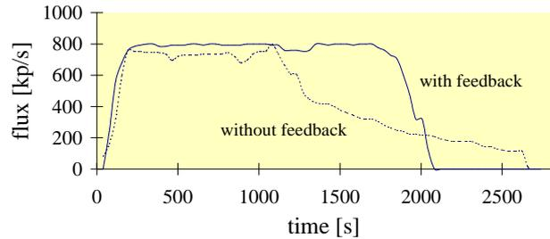
Figure 5: Spill from unstable machine
