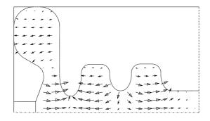
Figure 2:  $\pi$ -mode (f=2998.5 MHz) in the new design.
