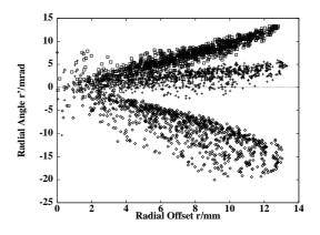
Figure 1: Transverse phase space plot of the first, middle and last bunch behind the solenoid (3  $TM_{01}$  cells).
