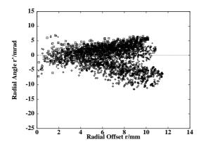
Figure 7: Transverse phase space of the first, middle and last bunch behind the solenoid (New design), E=100 MV/m.
