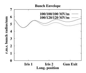
Figure 6: Evolution of the bunch radius in the gun for different accelerating gradients.
