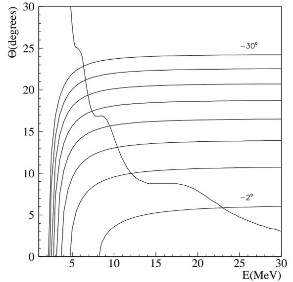
Figure 4: Lines of equal RF-phase difference at first section entrance.
