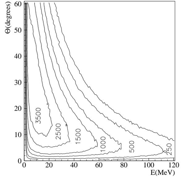
Figure 1: Lines of equal positron density. Tungsten, 2.5 radiation lengths.  $10^7$  incident electrons.
