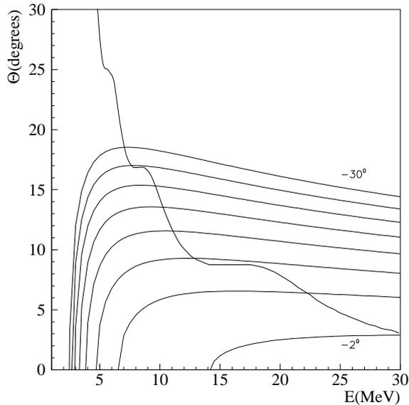
Figure 5: Lines of equal RF-phase difference after first accelerator section for fixed phase of accelerating field.
