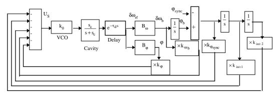
Fig. 6 Synchronization loop
