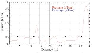
Fig. 3. Pressure profile, upstream interaction region
