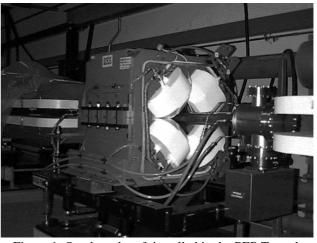
Figure 1. Quadrupole raft installed in the PEP Tunnel
