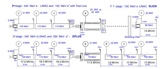
Figure 1 : Layout of the three building stages 1) ELIOS, 2)  $e^+$  Test line, 3) EPLUS
