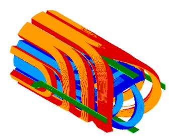
Figure : 2. MBCX-magnet lead end from ROXIE. Note the modelling of cross-over conductors
