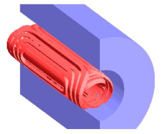
Figure : 3. MBCX-magnet Opera-3D® model. Only the return ends modelled for simplicity.
