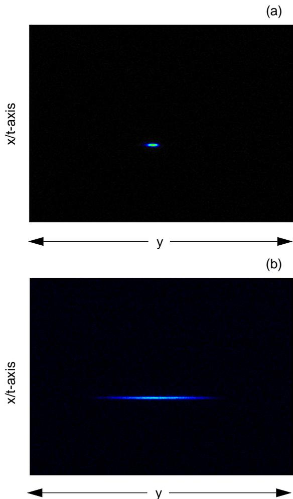
Figure 4: Focus-mode streak camera images showing the change in  $y$ -profile (displayed on the horizontal axis) without (a) and with (b) the induced head-tail instability.
