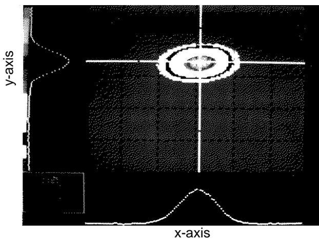
Figure 2: OSR image of the stored beam transverse beam sizes. The beam sizes are consistent with the 8.2 nm-rad natural emittance, assuming the lattice constants are within 10% of other design objectives.
