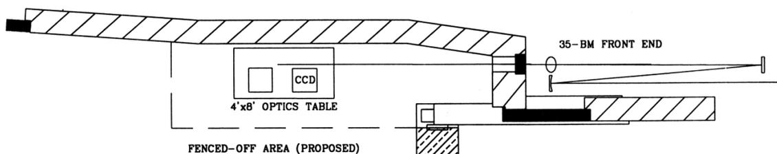
Figure 1: Schematic of the transport line for the UV-visible synchrotron radiation imaging station.
