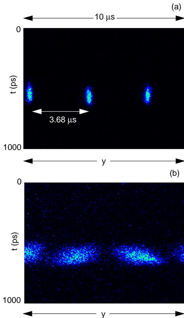
Figure 5: Dual-sweep mode streak camera images showing the change in the  $y$ - $t$  profile without (a) and with (b) the vertical instability.
