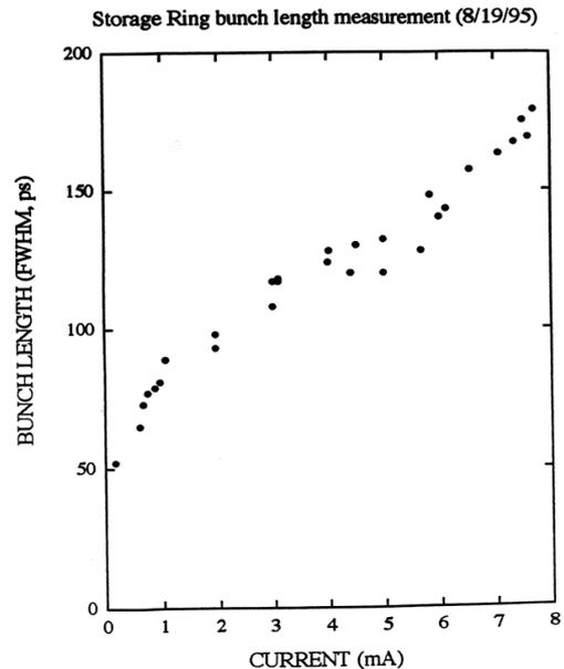
Figure 3: The observed bunch length versus single-bunch current as determined from streak camera measurements.
