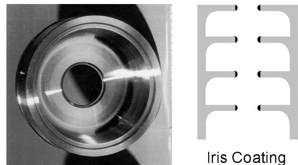
**Figure 3:** Picture of the iris coating to introduce losses for the HEM<sub>11</sub> mode with only little effect on the accelerating field.
