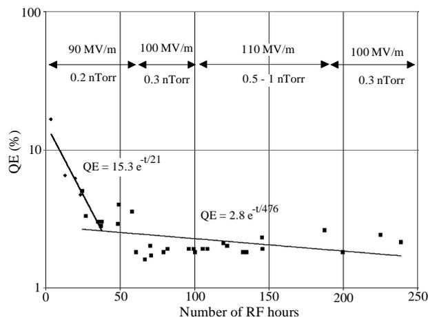
Figure 2. Quantum efficiency of Cs<sub>2</sub>Te cathodes as a function of RF hours. During the use of this cathode different RF field levels were applied as indicated.
