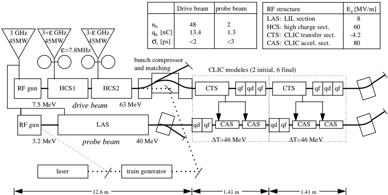
Figure 4. Sketch of CTF2. BPM's and focusing is omitted, except of the quadrupoles in the CLIC modules.
