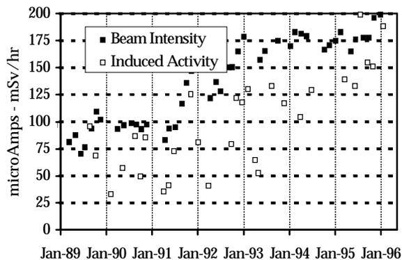
Figure 1. Average beam intensity/induced activity.
