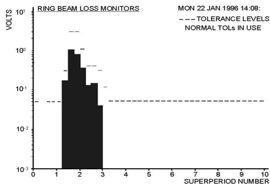
Figure 2. Prompt beam loss in the synchrotron.
