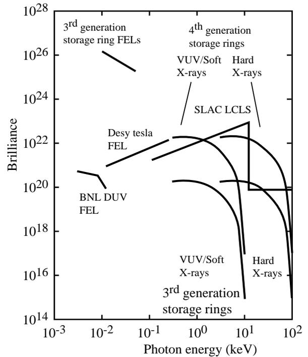
Fig. 2 - Average spectral brilliance [photonsxs<sup>-1</sup> mm<sup>-2</sup> mrad<sup>-2</sup> (0.1% Bandwidth)<sup>-1</sup>] of third and fourth generation Storage Rings compared with FEL performances (from Ref. [18] p. 21)
