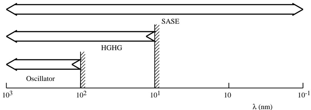
Fig. 1 - Operating regions for FEL oscillators, high gain harmonic generation devices (HGFG) and self amplified spontaneous emission devices (SASE)
