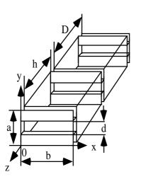
Figure 1: A rectangular accelerating structure
