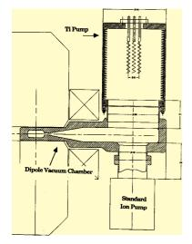
Figure 3: Final full scale prototype of DA $\Phi$ NE TSP-SIP pumping station and Dipole vacuum chamber.
