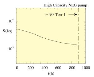
Figure 5: The result of the test on the final configuration of the DA $\Phi$ NE High Capacity NEG is reported. The pumping speed S (1/s) vs. time is shown. The testing conditions relate 900 hr to  $\approx$  90 Torr l of pumped gas.
