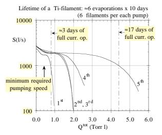
Figure 4: The pumping speed S (l/s) of the DA $\Phi$ NE TSP with one Ti filament is reported vs. the total pumped gas load Q<sup>tot</sup>(Torr 1). Each filament allows 6 sublimation covering  $\approx 60$  days of full current operation (after conditioning). Each TSP cartridge provides 6 filaments.
