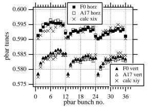
**Figure 2** : Measured and Calculated Pbar Tunes for Colliding Beam Conditions. We assume base pbar horizontal and vertical tunes of 0.5855 and 0.5755, horizontal proton emittances equal to the vertical proton emittances, and we use a scale factor of 0.648 for the tune shifts from the head on beam beam interaction.
