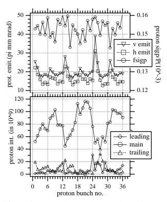
**Figure 1** : Bunch by bunch proton intensities and emittances at 900 GeV in colliding beam conditions.
