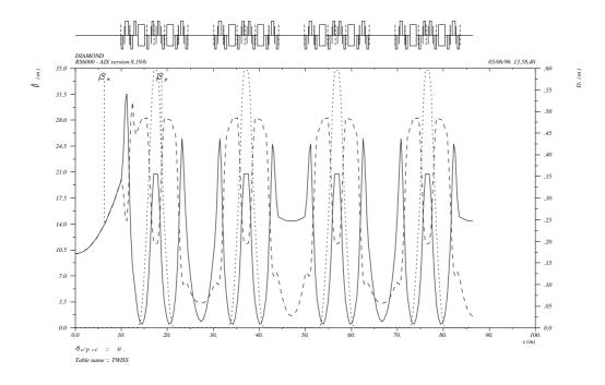
Figure 1: Optical functions for a quarter of DIAMOND.
