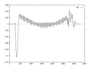
Figure 3: Relative transverse displacement of LHC in meter, between IP1 and IP8
