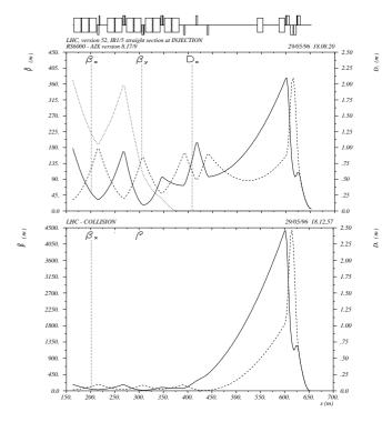
Figure 4: Insertion optics at injection and in collision
