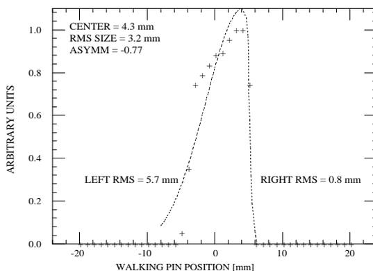
Figure 2: Vertical scan of  $^{40}\text{Ar}^{11+}$ .
