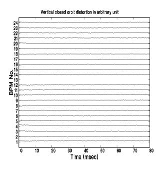
Fig. 2 Vertical closed orbit distortion during ramping when all 3 extraction bumpers were turned off. The distance between two ticks is 15 mm. The tick marks on both sides also mark the ideal orbit of the corresponding BPM.
