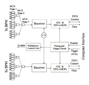
Fig. 1 Block diagram of the electronic hardware
