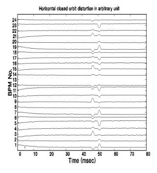
Fig. 4 Horizontal closed orbit during ramping when the first bumper and the third bumper were turned on, and the timing was separating by 4 msec. The distance between two ticks is 15 mm. The tick marks on both sides also mark the ideal orbit of the corresponding BPM.
