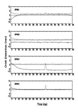
Fig. 3 The horizontal and vertical beam closed orbit distortion during ramping. The extraction bumpers were turned on with the routine operation condition. In the figure the horizontal beam positions are connected by solid line, and the vertical beam positions are connected by dotted line.
