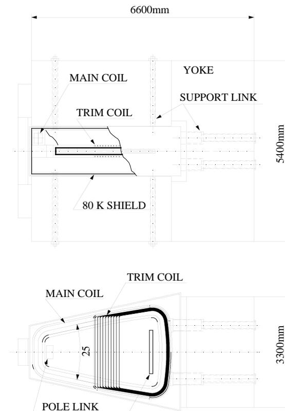
Fig. 1 A schematic drawing of the model sector magnet: a side view(upper); a top view(lower).
