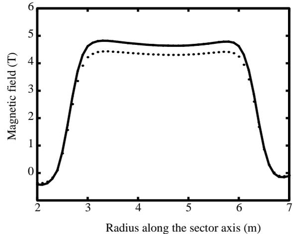
Fig. 3 Calculated median-plane field distributions along the central line of sector magnet. The solid and dotted lines show the distributions at the ampere-turn of 6 and 5.25 MA, respectively.
