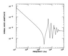
Figure 4: Calculated normal-mode admittance of the BSR dipole magnet strings
