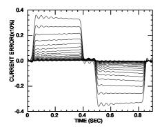
Figure 3: Current-pattern errors during the self-learning process
