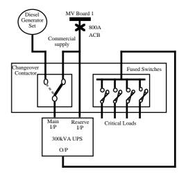
Figure 1: UPS Connection Diagram
