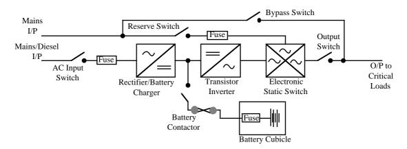
Figure 2 : UPS Circuit Diagram
