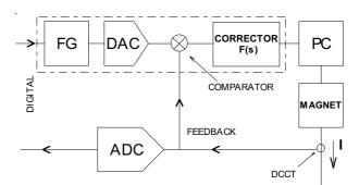
Fig 1 Typical Analogue Control Loop
