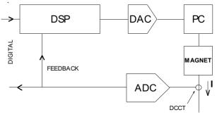
Fig 2 Basic Digital Control Loop
