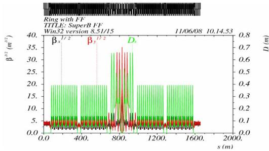
Figure 1: LER optical functions.
