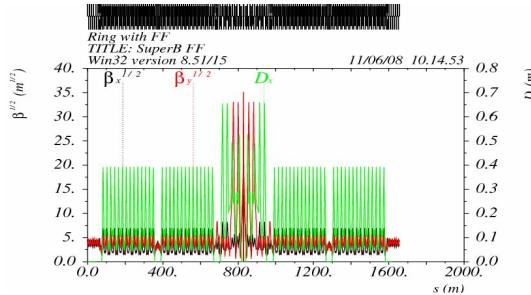
Figure 1: LER optical functions.
