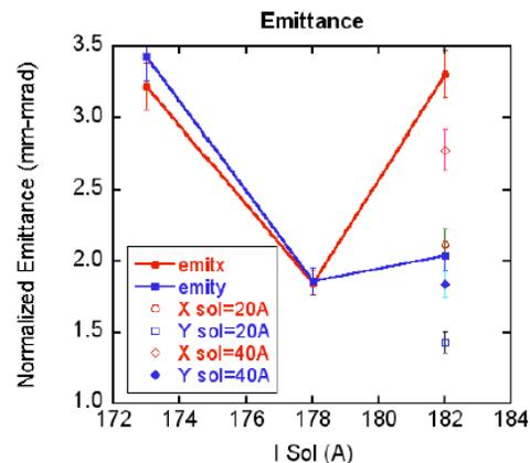
Figure 3: Emittance measurement for different configuration of the gun solenoid and the coils around the accelerating structures.
