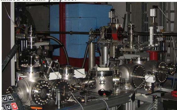
Figure 5: Harmonic generation chamber in the SPARC Hall.
