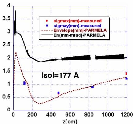
Figure 4: PARMELA simulation of the envelope and emittance corresponding to the best measurement shown in Fig. 3. The measured envelopes (blue rectangle) are also shown.
