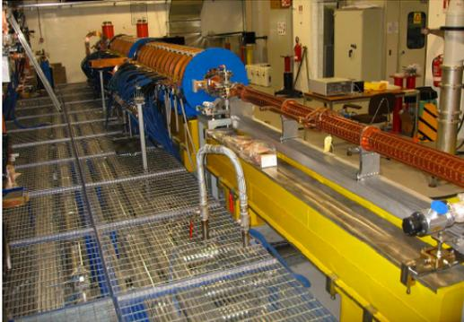
Figure 1: Picture of the SPARC photoinjector showing 13 accelerating structures with 2 long solenoids.
