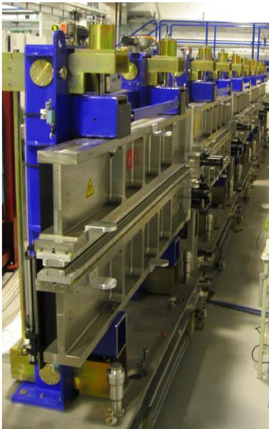
Figure 2: Picture of the SPARC undulator chain during installation.
