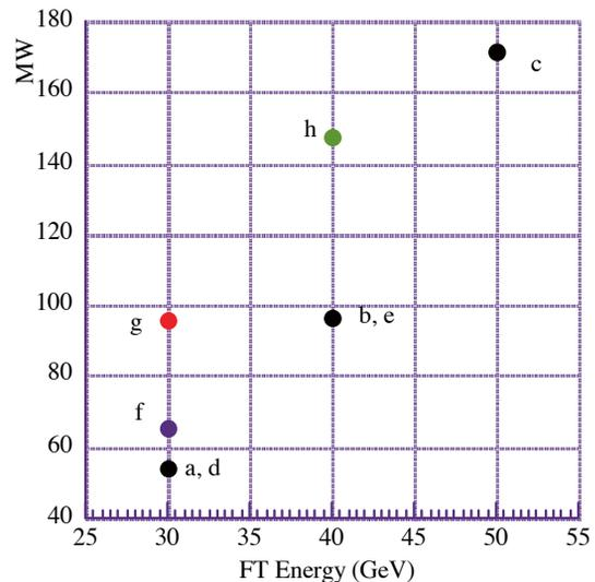
Figure 3: Total pulse power amplitudes for the various patterns as shown in Table 1. The disturbance level is allowable if the total pulse power amplitude is less than 100 MW, such as pattern a, b, d, e, f and g. However, pattern g requires the power supply upgrade. Patterns c and h require both of power supply upgrade and some energy storage system.
