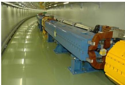
Fig. 4: Bending magnets and quadrupole magnets installed in the MR tunnel.
