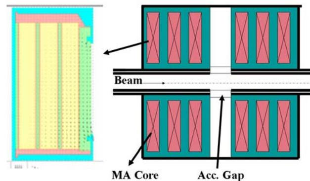
Fig. 7: Schematic cross sectional view of accelerating cavity (right) and calculated field distribution (a quarter) in the cavity are shown.
