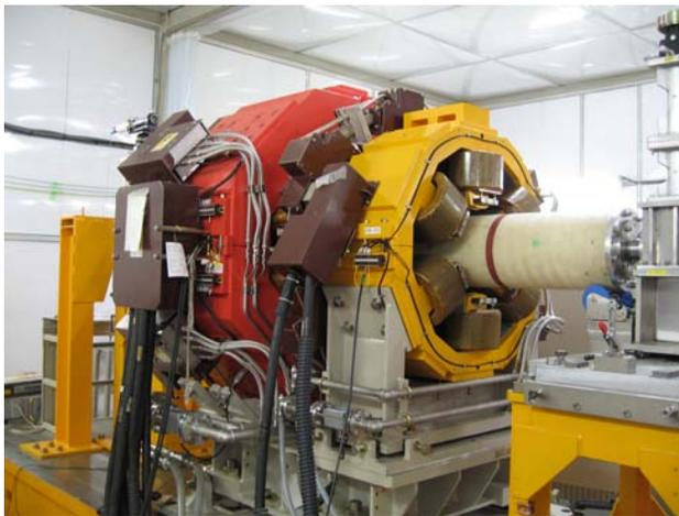
Fig. 6: Measurement of magnetic field interference between a quadrupole and sextupole magnet.
