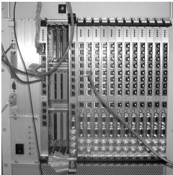
Figure 1: The 9U VME chassis for dual harmonic signal synthesis.
