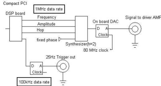
Figure 3: DSP+DDS Combination for high power tests.
