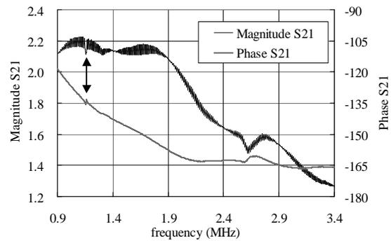
Figure 6: S21 transfer function of the RCS high power system measured between driver amplifier input and differential signal of both capacitive gap voltage dividers.
