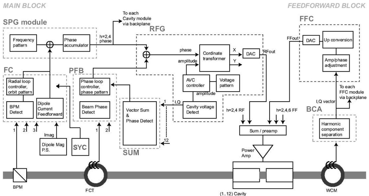
Figure 2: Block diagram of the RCS LLRF system [5]. The elements marked in green exist once. The elements marked in red exist 12 times.
