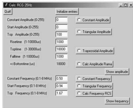
Figure 4: GUI for calculation of acceleration patterns.
