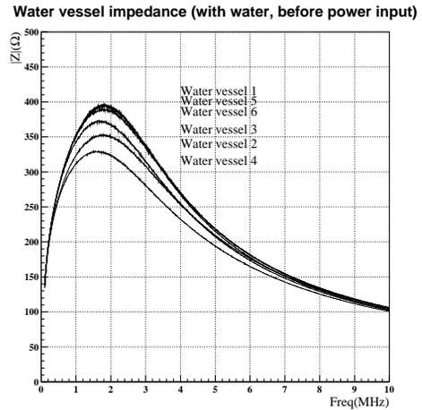
Figure 2: The magnitude of the impedance  $|Z|$  of the cores stacked in the water vessel.
