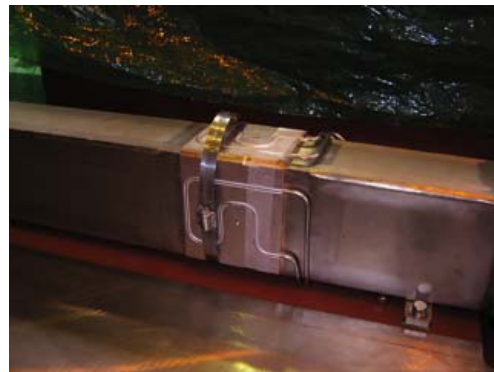
Figure 9: Cooler panel is bonded on the collimator duct.
