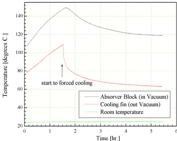
Figure 4. Cooling test at 700 Watt heating
