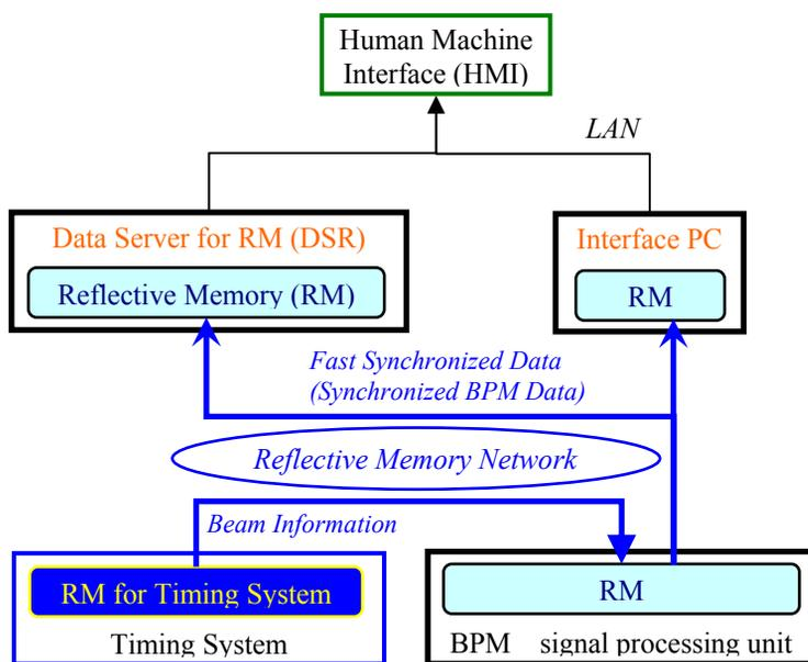
Figure 2: BPM data collection system configure
