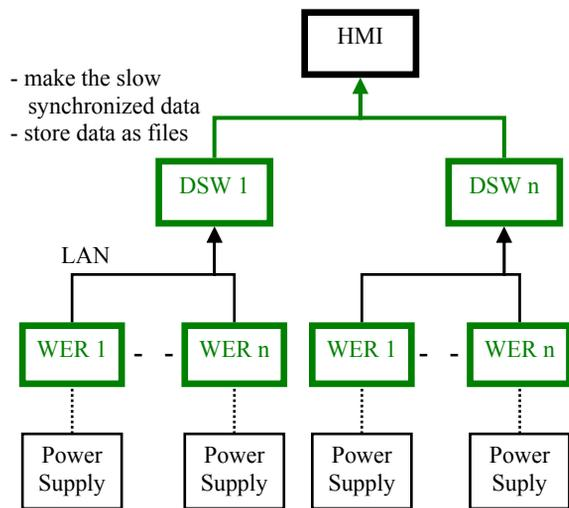
Figure 5: Configure of slow synchronized data monitoring and acquisition system
