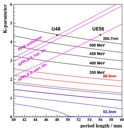
Figure 2: K-parameters for various undulator designs compared to K-parameters needed to generate 266.7 nm, 88.9nm and 53.3nm radiation for electron energies between 350-500MeV.
