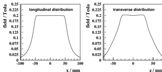
Figure 3: Longitudinal and transverse field distribution of one chicane magnet.
