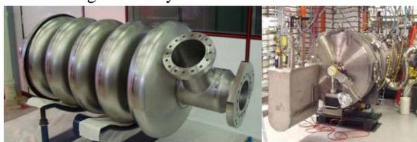
Figure 6. The 5-cell,  $\beta_0=0.65$  CEA/CNRS cavity and the SNS cryomodule.
