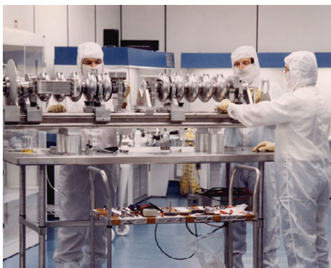
Figure 1: Clean room final assembly of a CEBAF cavity pair at TJNAF.
