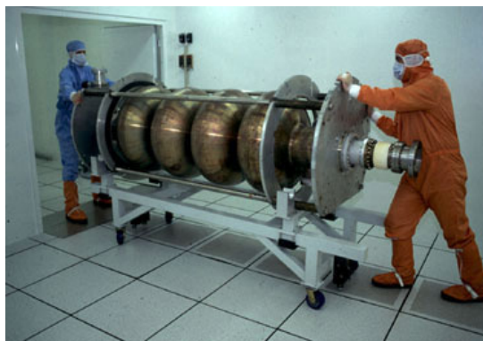
Figure 2: One of the 352 MHz LEP II cavity at one step of the clean room handling in industry.
