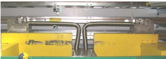
Figure 3: Double Contained Co-Axial Piping System
