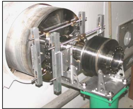
Figure 9: Co-Axial Bellows & Vacuum Clamp Assembly
