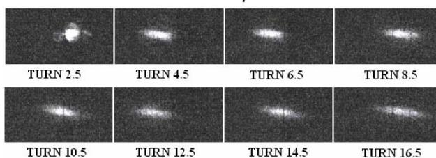
Figure 3: Beam spot produced by the extracted  $H_2^+$  beam on the phosphor screen situated above the median plane. The peak beam current was approx 20  $\mu A$ , beam energy 20 keV, and a pulse length 1  $\mu sec$ . Each frame is approximately 60 mm by 30 mm.
