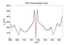
Figure 1: LER (top picture) and HER (bottom picture) vertical beam size as computed with MAD (blue line) and AT (red line).
