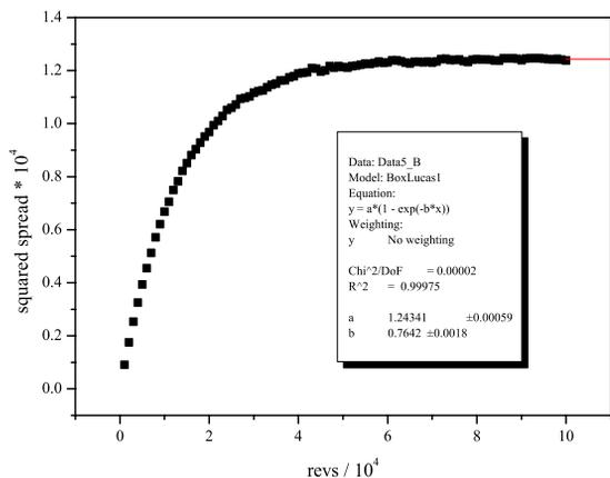
Figure 1: Temporary behavior of energy spread. Number of particles  $10^5$ , probability of interaction per rev 0.1
