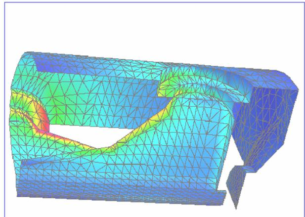
Figure 2: Finite elements model of the end cell in "OPERA - 3D" code
