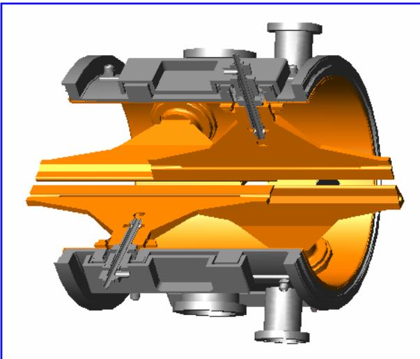
Figure 4: The regular cell of the RFQ.
