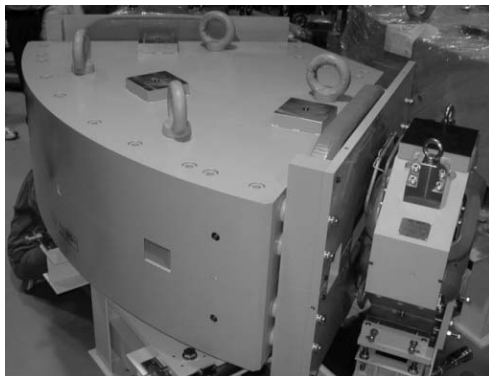
Figure 2: One unit of the bending magnet and the quadrupole magnets.
