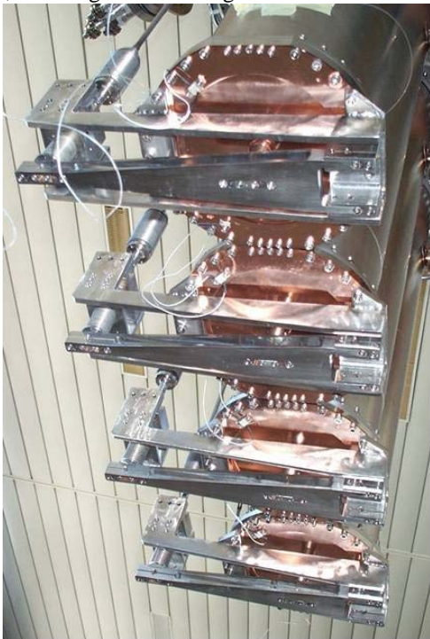
Figure 6. New tuners mounted in resonators ready for installation in the linac.
