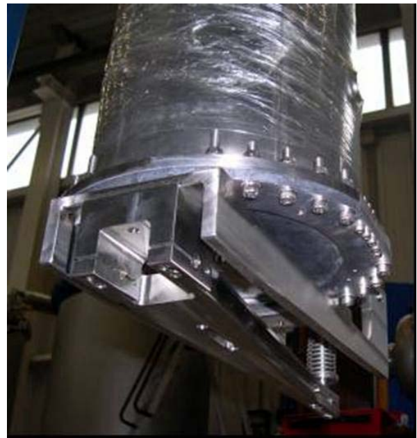
Figure 4. The new tuner prototype #1, mounted on a 80 MHz resonator
