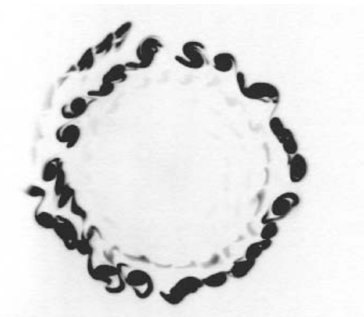
Figure 3: Vortex and hollow beam formation, before B_0 = 500 G is decreased slowly, with j_{th} = 2.2 A/m 2 , and L = 1.1 m; full movie at Ref. [7]
