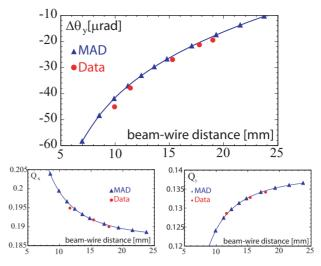
Figure 3: Closed-orbit deflection angle at the wire fitted from the nearby BPM readings (top) and the measured horizontal (bottom left) or vertical betatron tune (bottom right) as a function of the beam-wire distance compared with MAD predictions; for a wire current of 267 A at 55 GeV/c.
