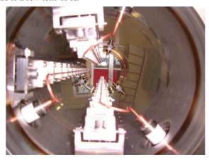
Figure 1: Photo of a new 3-wire device during assembly.
