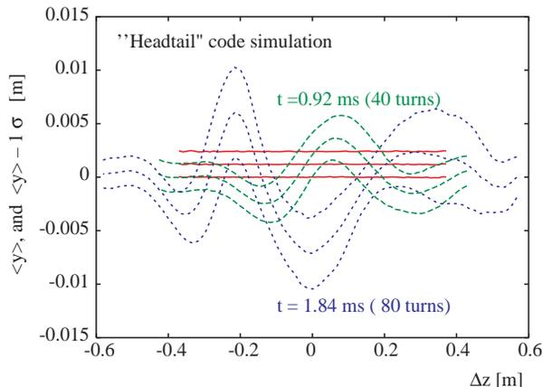
Figure 4: Vertical centroid with  $\pm 1\sigma$  bands at injection (red), and 40 and 80 turns later.
