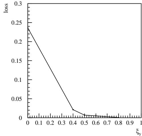
Figure 2: Fraction lost in the first 10 ms as function of the vertical chromaticity  $\xi_y$ . Injection at 0.6 MV,  $\epsilon_l = 0.2 \text{ eV s}$ ,  $4\sigma_t = 2.7 \text{ ns}$ .
