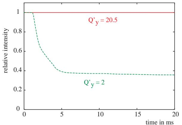
Figure 3: Simulation using the "Headtail" code. Relative intensity in the first 20 ms following injection of  $1.2 \times 10^{11}$  protons for low and high chromaticity.
