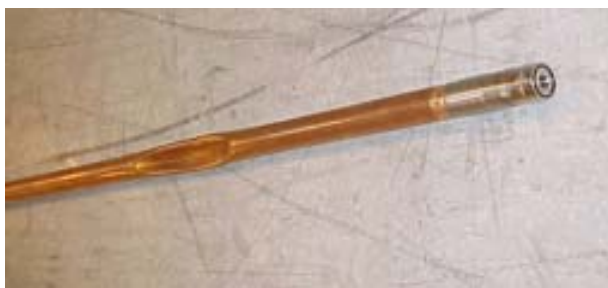
Figure 3: full-scale destructive test, buckling mode
