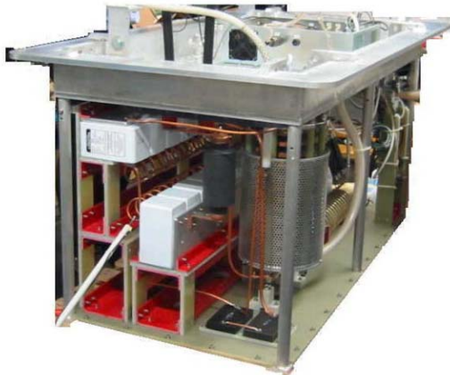
Figure 3: High voltage modulator internal portion.
