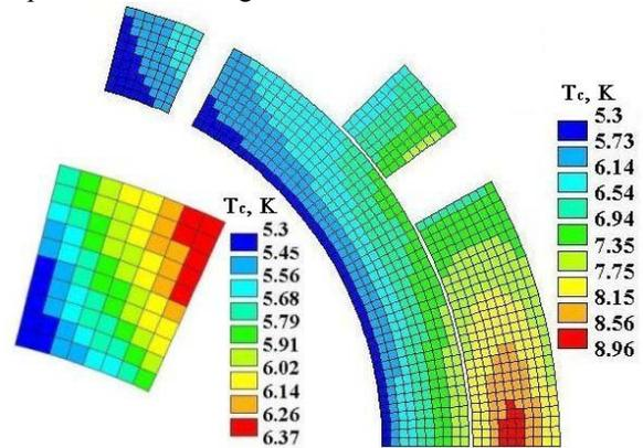
Figure 4. Distribution of the critical temperature in the coil for the design II of SC dipole.
