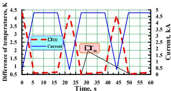
Figure 6. Difference between critical and operating temperatures for the last turn of the inner layer.
