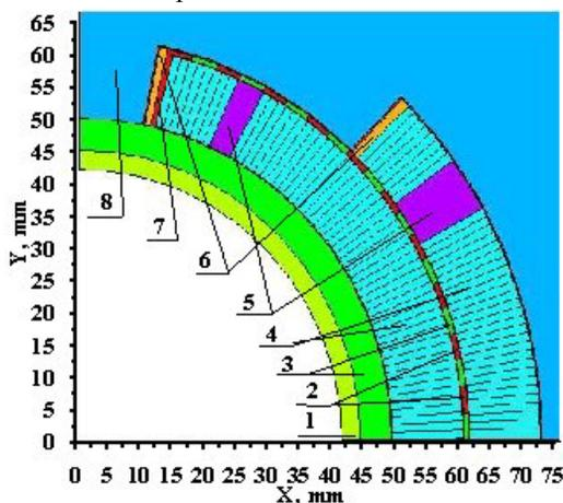
Figure 1. Cooling scheme of the SC dipole in the cross section: 1 - beam pipe, 2 - glass-cloth laminate spacers of helium channels, 3 - helium channels, 4 - coil, 5 - inter-turn spacers, 6 - shims, 7 - spacers for helium channels, 8 - collars.
