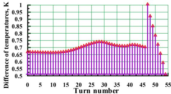
Figure 8. Minimal difference between critical and operating temperatures in turns of the inner layer.
