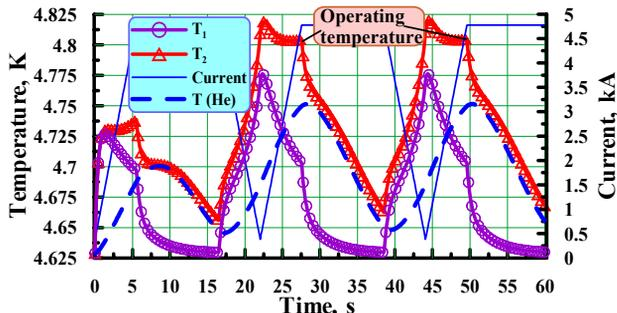
Figure 5. Temperature in the last turn of the inner layer in the last dipole of the string: thick violet line (o) shows temperature  $T_1$ , where is an inlet helium, thick red line ( $\Delta$ ) shows the temperature  $T_2$  in the place of outlet helium. Blue dashed line shows the temperature  $T(He)$  of outlet helium from the last dipole in the string and thin blue line shows the operating current.
