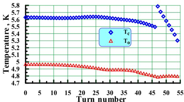
Figure 7. Critical ( $T_c$ ) and operating ( $T_o$ ) temperatures in turns of the inner layer corresponding  $\Delta T_{min}$ .
