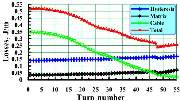
Figure 2. AC losses per cycle in turns of the inner layer (the first quadrant).
