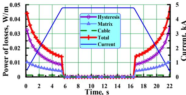
Figure 3. Power of losses in the last turn of the inner layer and operating current versus time of cycle.
